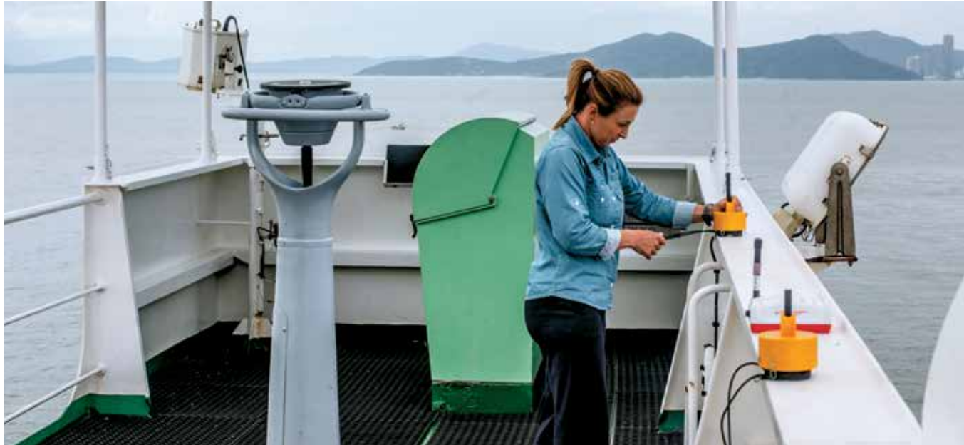
PILOT LIVIA LAGE INSTALLING PPU ANTENNAS ON THE SHIP'S BRIDGE WING
