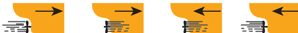
Figure A2. The four quadrants of the propeller a) ship going ahead and propeller rotating in the design direction; b) ship going ahead and propeller rotation inverted; c) ship going astern and propeller rotation inverted; d) vessel going astern and propeller rotating in the design direction (Harvald, 1977, apud PIANC,1992, Bulletin 77 )
